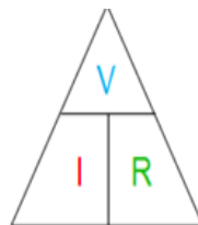
Figure 1.4.2 : Ohms Law Triangle
